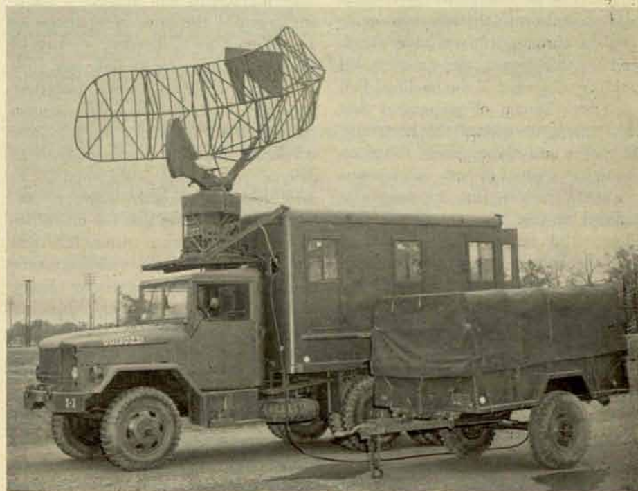
Converted mobile AN/TPS-1D radar set and repair van, 71st AAA Battalion.
