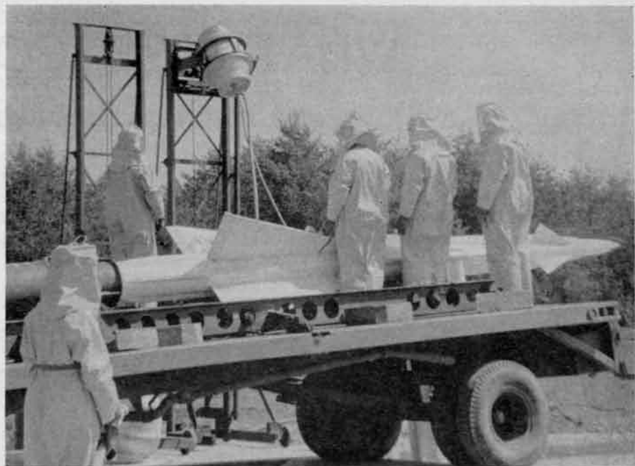
Captain Vanture (right) and crew in "Men from Mars" costume prepare to pour acid from drum to missile tank.
